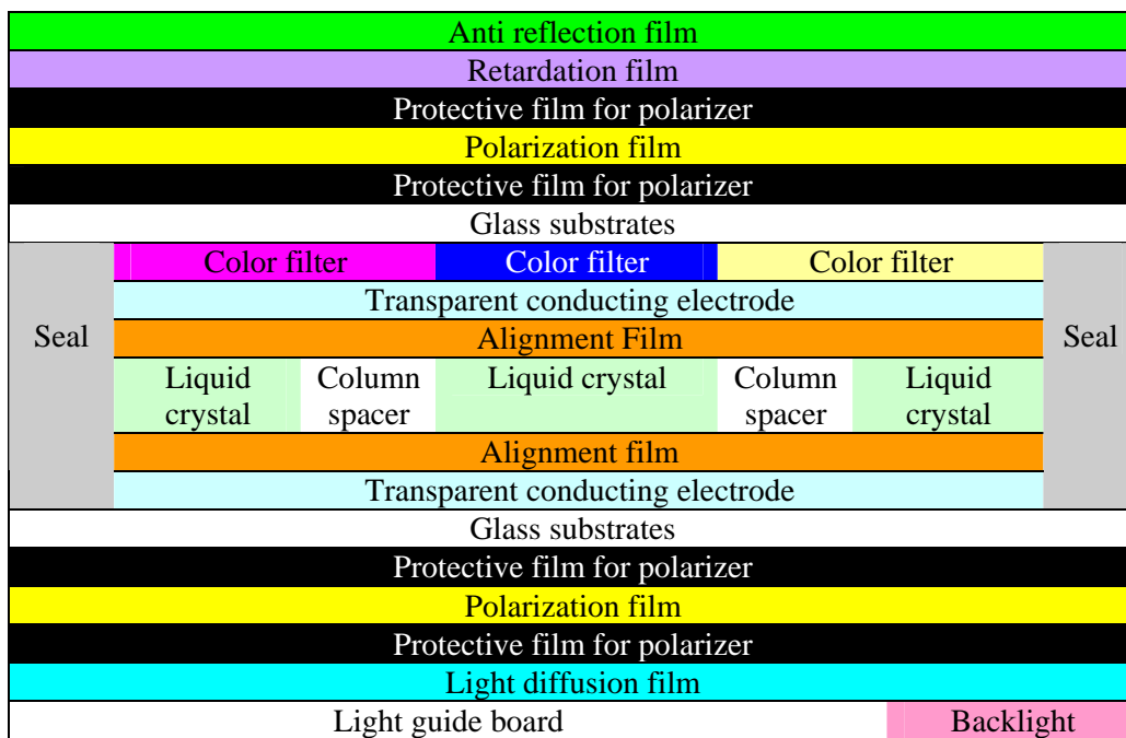
Figure-2: Main Materials Composing LCD
